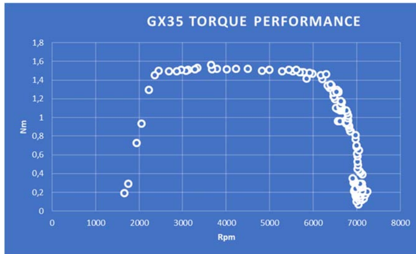
Figure 8 Results from testing the Honda Gx35 engine on the dynamometer
