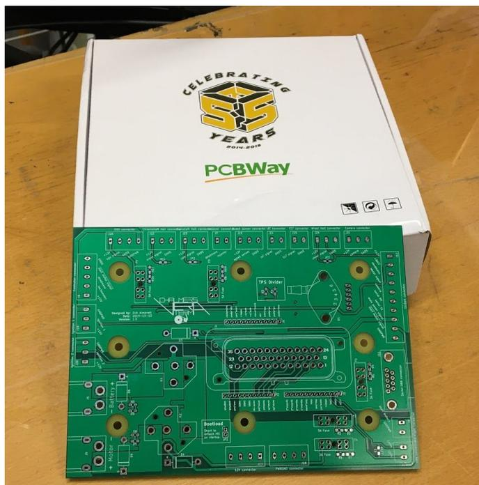
Our vehicle, Vera III, have several integrated system with PCBs and now we wanted to create the mainboard. It is mostly a power distribution board and connects the ECU and all sensors in a clean and simple way. It is also a connector for the engine starter and other subsystems. The board has to be high quality to be able to handle the environment and the high power consumption of the start engine. The ambient temperature is probably over 60 degrees celsius and a constant vibration.
